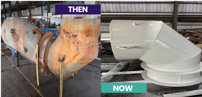
Seawater Condenser Pipe Elbows for Units 5 and 6 of the San Juan Power Plant.
