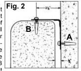
component C away from the wall to drill, molly and screw the bracket against the wall as shown in Fig. 2 (A). With bracket in place, reposition component C and drill, molly and screw the bracket to wall component Fig. 2 (B).
